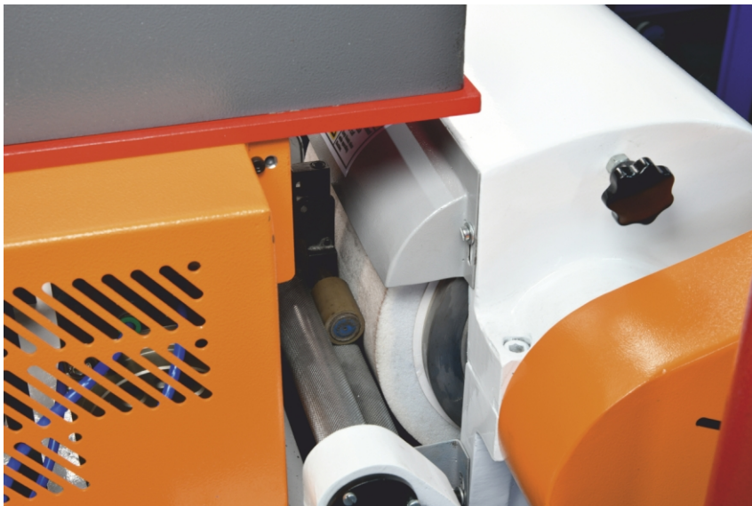
Fully automatic grinding of speed frame cots
