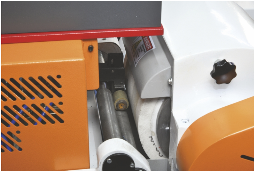
Fully automatic grinding of ring frame cots
